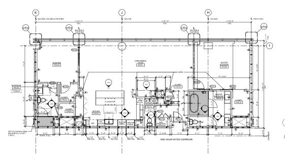
LEGEND NOTE: CONTRACTOR SHALL BE RESPONSIBLE FOR COORDINATING AND MAINTAINING THE COOR-REQUIRED MIN. CLEAR WIDTH IN KITCHENS, AS DESCRIBED IN SECTION 1133A 2.A OF THE 2013 CBC (TYP., U.O.N.)
